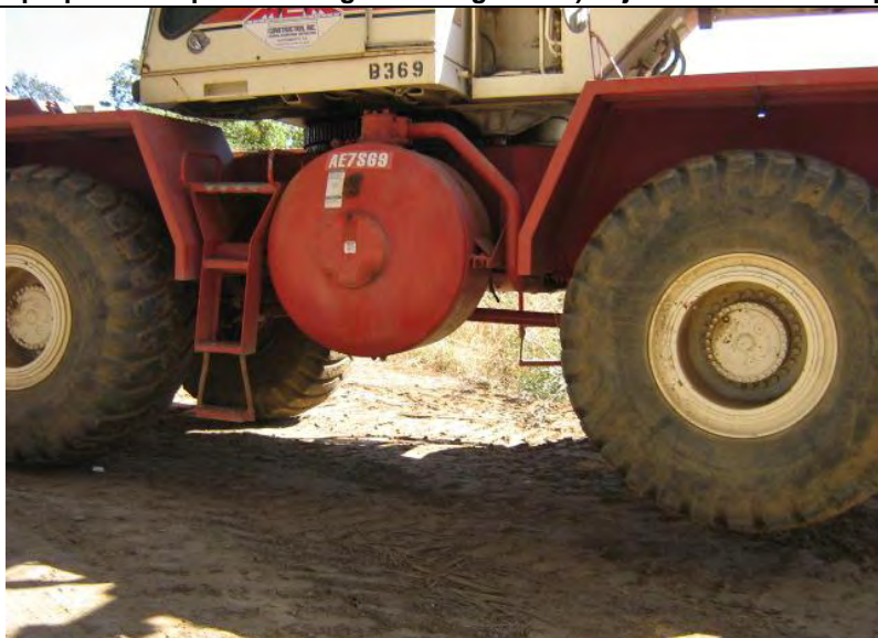
Photograph 3 – Equipment with petroleum product leaking onto ground surface (see Photograph 4 for close-up view).
