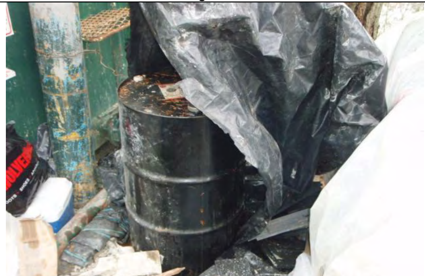
Photograph 8 – 55-gallon drum of "Rock Drill 150" that is partially covered and not within adequate secondary containment
