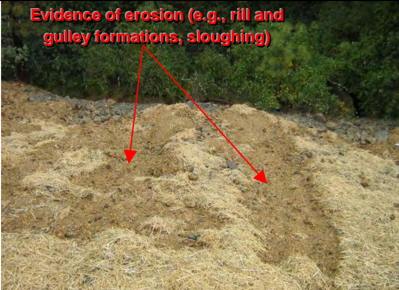
Photograph 3 – Evidence of erosion (e.g., rill and gully formation) and sediment transport from the disturbed slope failure
