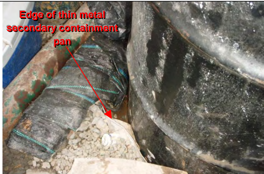
Photograph 9— Close-up view of damaged secondary containment pan underneath 55-gallon drum
