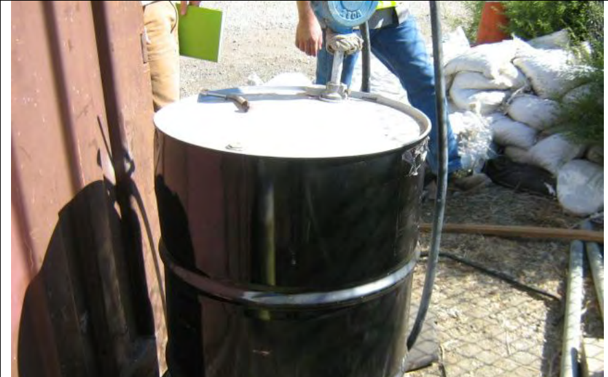
Photograph 6 – Asphalt release agent without secondary containment
