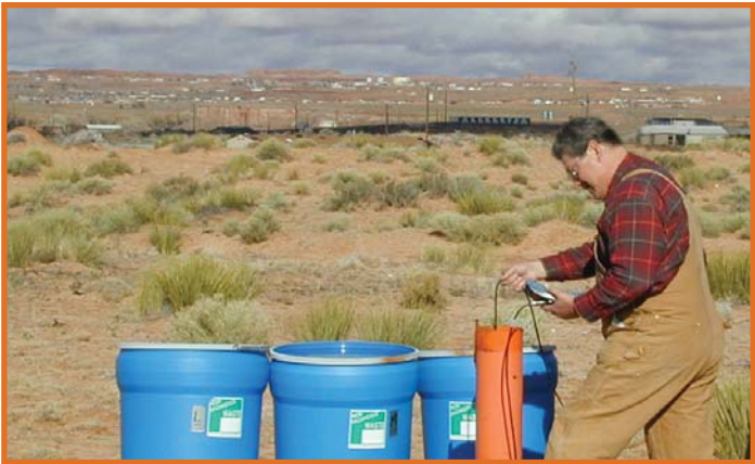
Pictured on the right: Data collection at a groundwater monitoring well near the Tuba City Open Dump site. As part of the site investigation currently underway at the Open Dump site, groundwater chemistry data is gathered to determine what contaminants may possibly be in the groundwater.
