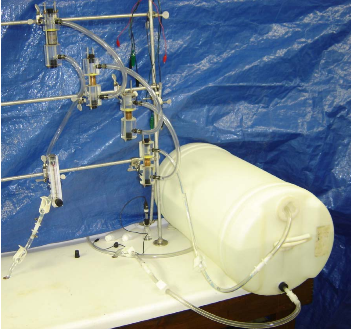
Figure 3. Photo of a pipe rig with indirectly-coupled cells in operation.
