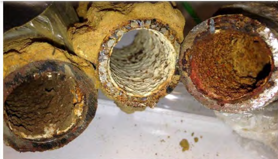
A view into Flint drinking water pipes, showing various types of iron corrosion and rust. (Min Tang and Kelsey Pieper)
