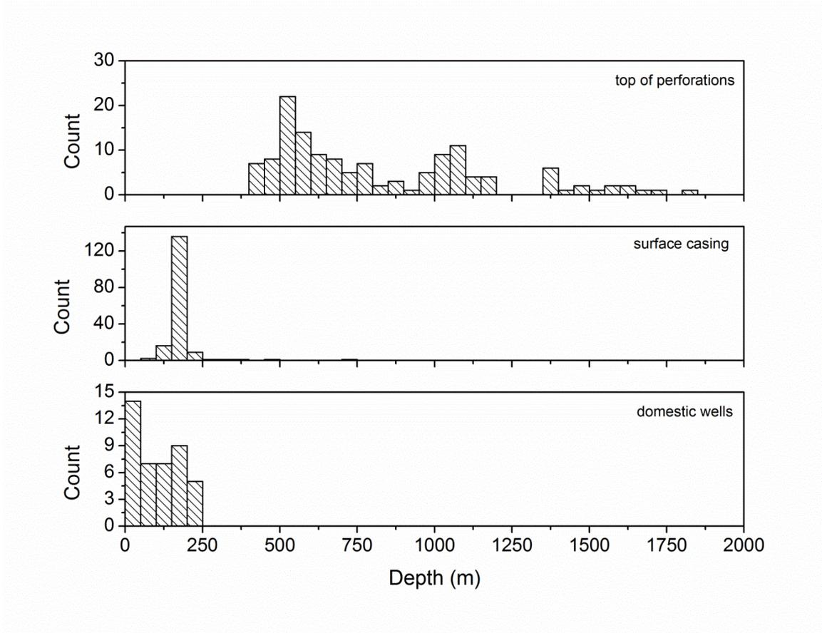
**Histograms summarizing depths of top of perforation interval of production wells, base of surface casing of production wells, and base of screened interval of domestic wells.**
