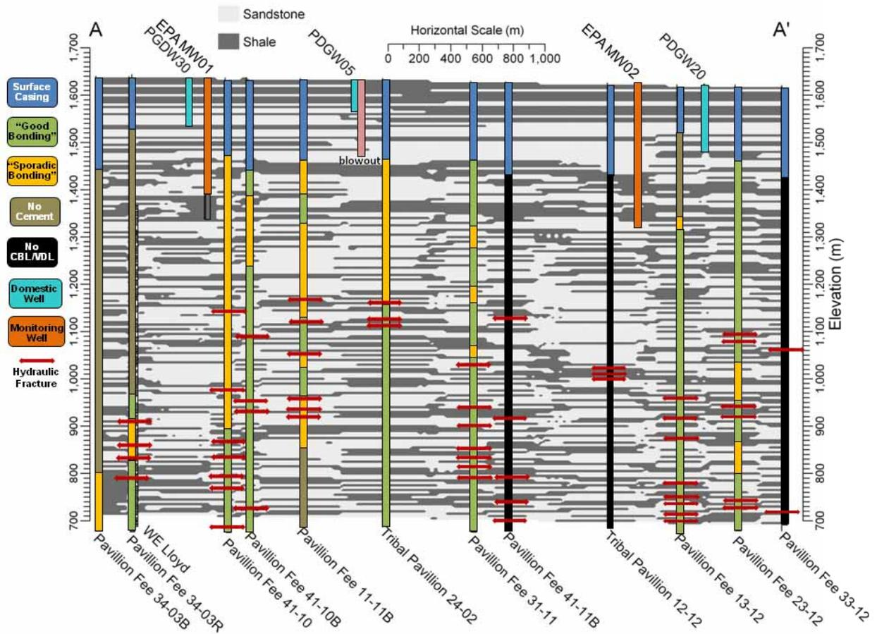
**Fig. 3b. Lithologic cross-section along transect illustrating production wells (with evaluation of CBL/VDLs), domestic wells, and blowout location. Red arrows denote depths of hydraulic fracturing of unknown areal extent.**
