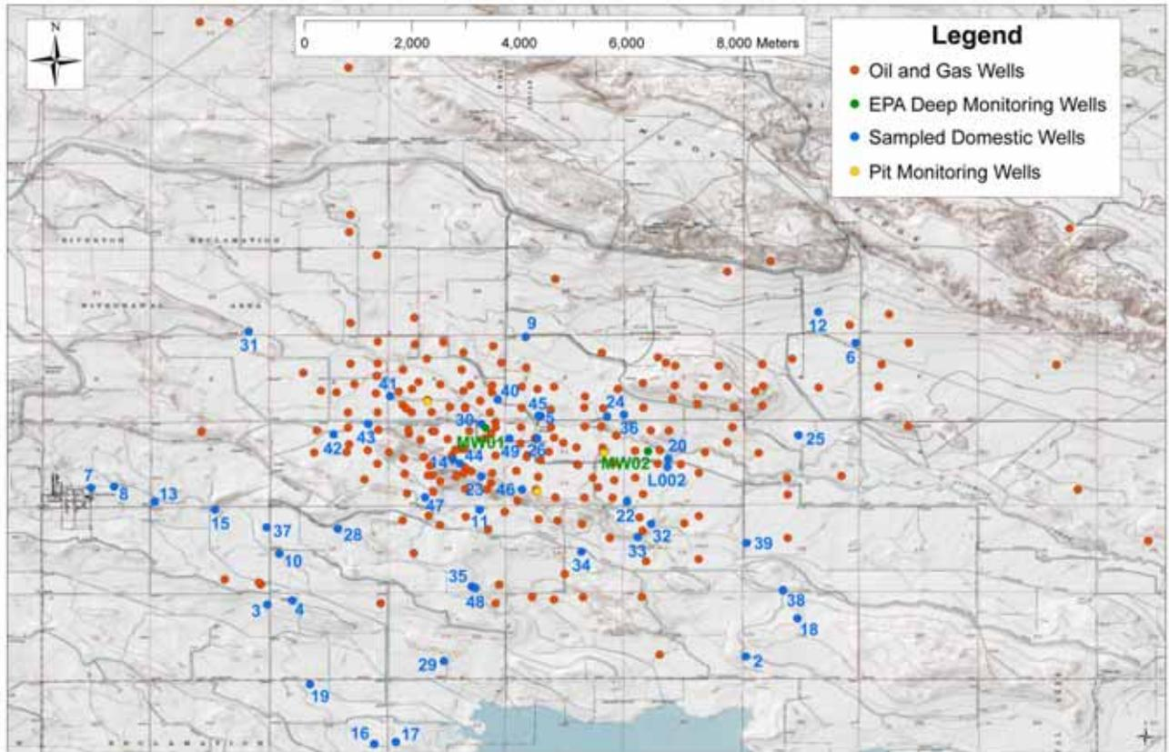
**Fig. 1. Map illustrating location of oil and gas production wells, sampled PGDW series domestic wells (only numbers shown to conserve space), two deep monitoring wells and three shallow monitoring wells near pits. PGDW07 and 08 are municipal wells in the Town of Pavillion.**
