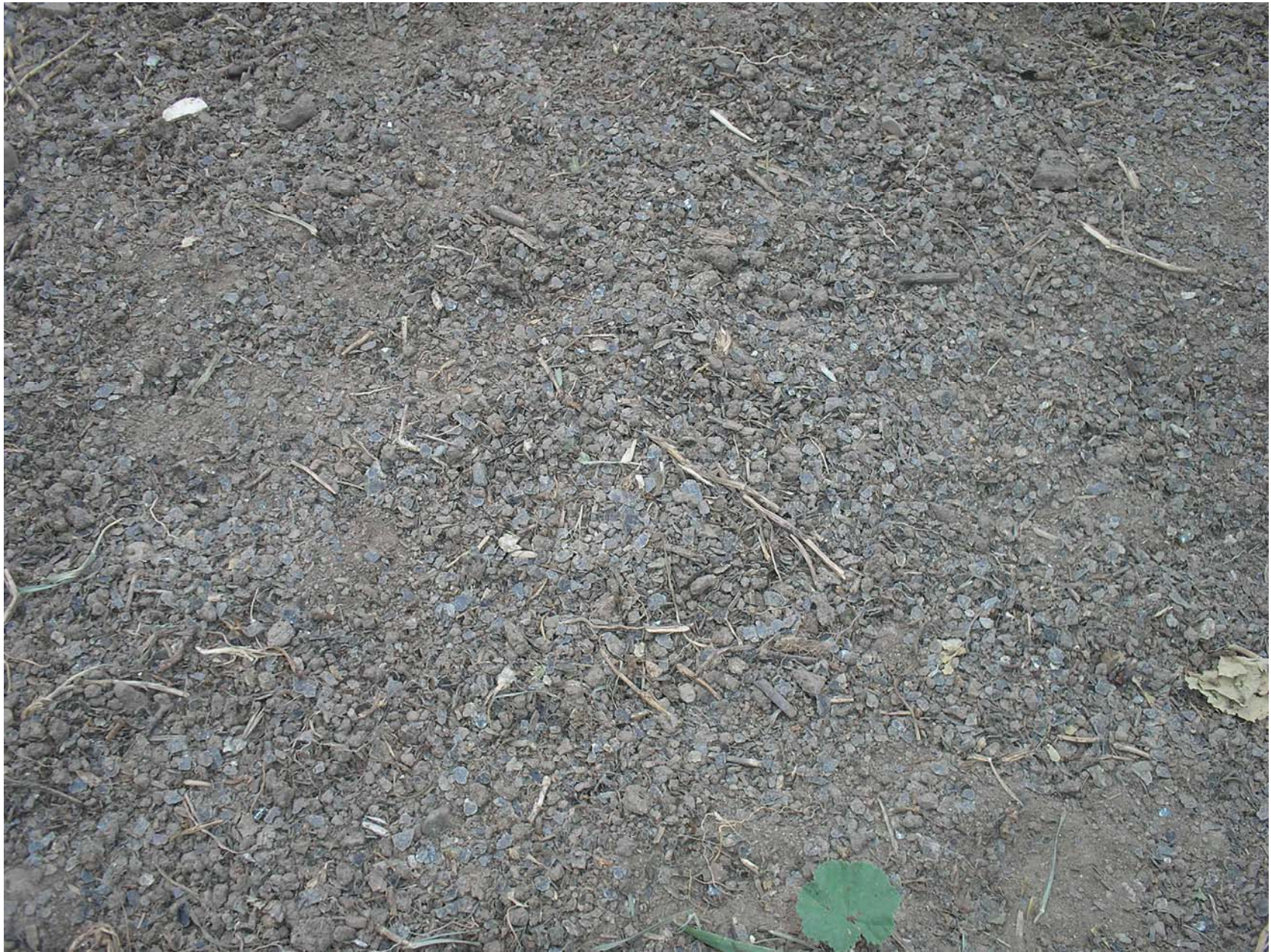
Figure 2d: High Visible Vermiculite – Vermiculite easily observed throughout visual inspection point, including the surface.
