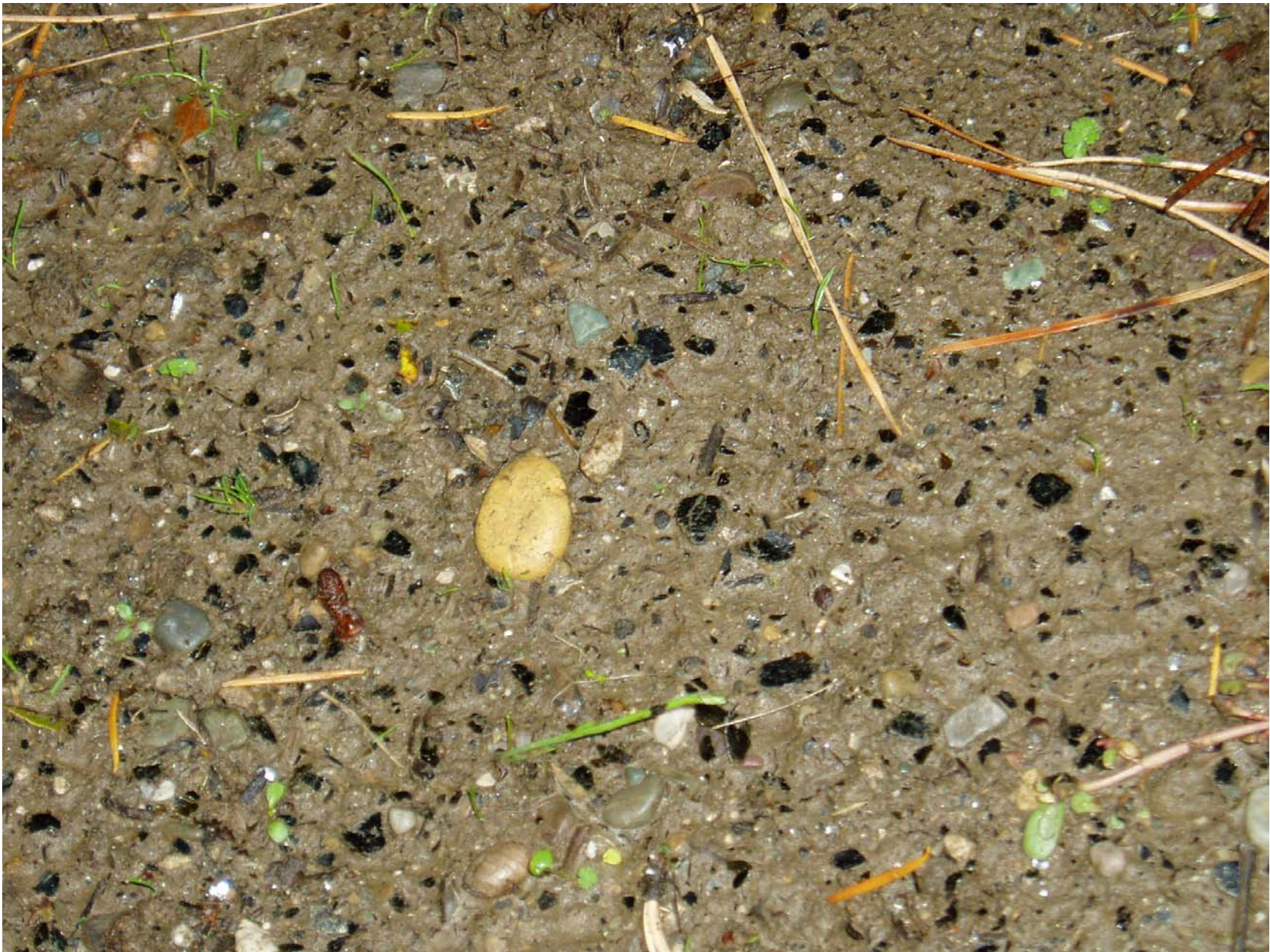
Figure 2c: Intermediate Visible Vermiculite – Vermiculite easily observed throughout visual inspection point, including the surface.
