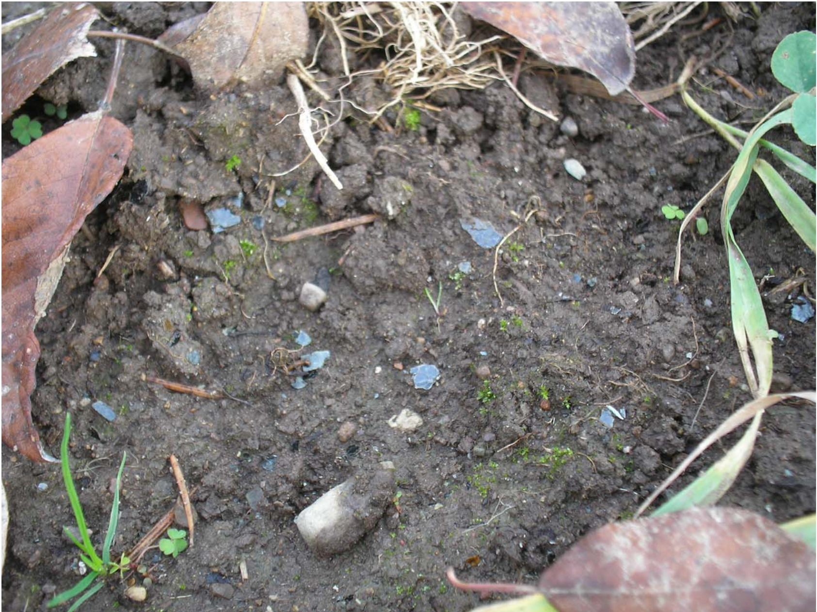
Figure 2b: Intermediate Visible Vermiculite – Vermiculite easily observed throughout visual inspection point, including the surface.
