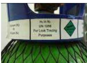
A trace of hydrogen or helium with the nitrogen will enable leaks to be found at a lower pressure. A suitable electronic detector must be used – your standard detector is not sensitive to hydrogen or helium. Nitrogen can be supplied with a trace of hydrogen (as shown in the photo) or helium specifically for leak testing.
