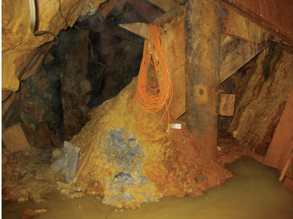
Figure 13. Ore chute with pile of mined material below, Standard Mine Level 3. Brown-colored material on pile primarily consists of goethite [ \text{FeO}(\text{OH}) ] and plumbojarosite [ \text{PbFe}_6(\text{SO}_4)_4(\text{OH})_{12} ] which are secondary iron-rich phases that form by the oxidation of sulfides. Gray color in photograph is exposed material below brown surface containing fragments of galena and quartz with minor pyrite as well as secondary lead mineral phases and goethite.
