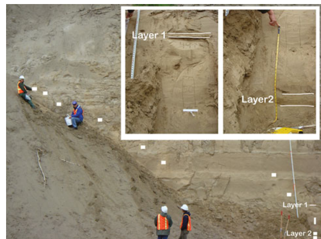
Fig. 12 Sample sites from clay pit (white boxes), and two sample localities containing LA (labeled). More detail is shown on the inset photos
