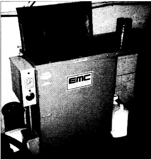
Glenmoor Auto Repair use a small, inexpensive spray cabinet which cost them $1,700. They send large parts off-site for steam cleaning.
