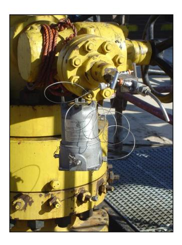
To facilitate doing long-duration tests, memory gauges are used to monitor and record the pressure fall-off downhole or more commonly at the wellhead.
