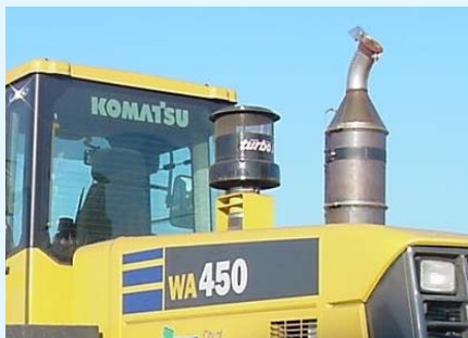
Front loader retrofitted with DPF. Image courtesy U.S. EPA 8
