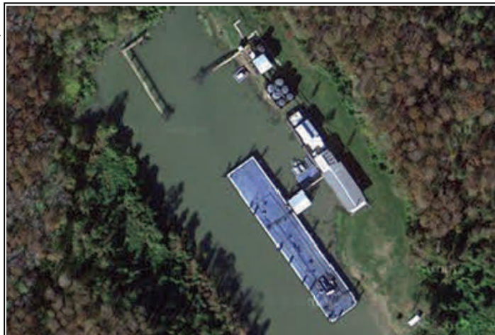
Aerial photograph of the overall well site at FAS with living quarters and a barge parked at the dock. Barges ferried wastewater from the FAS transfer station to the well site for disposal into the injection well.
