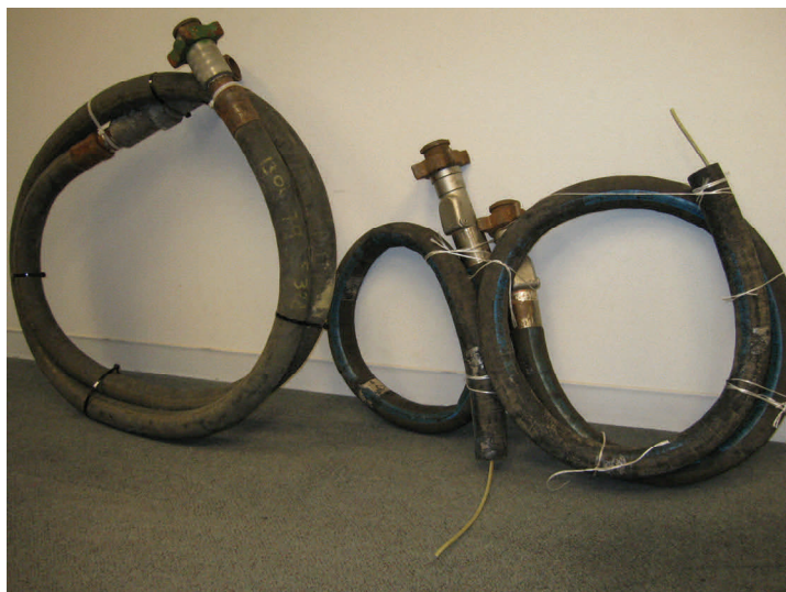
Hoses that were used during the anhydrous ammonia product transfer
