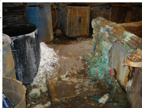
Vats, caustics and precipitate. Note the “drag out” from years of electroplating. Hazardous waste from the business had never been properly disposed of by the defendant, despite operating the company for over 14 years.
