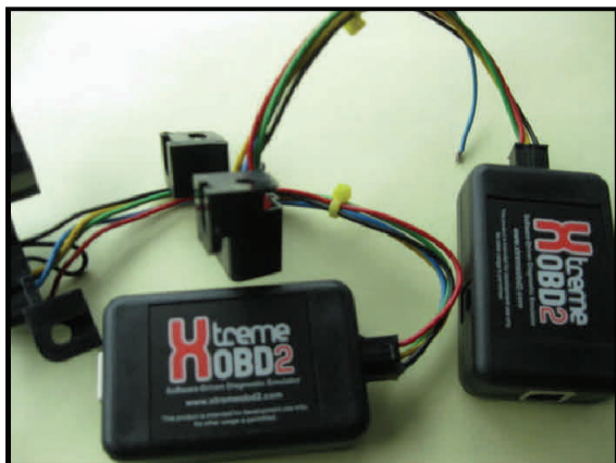
Example of an OBDII Simulator used by inspectors to bypass emission testing
