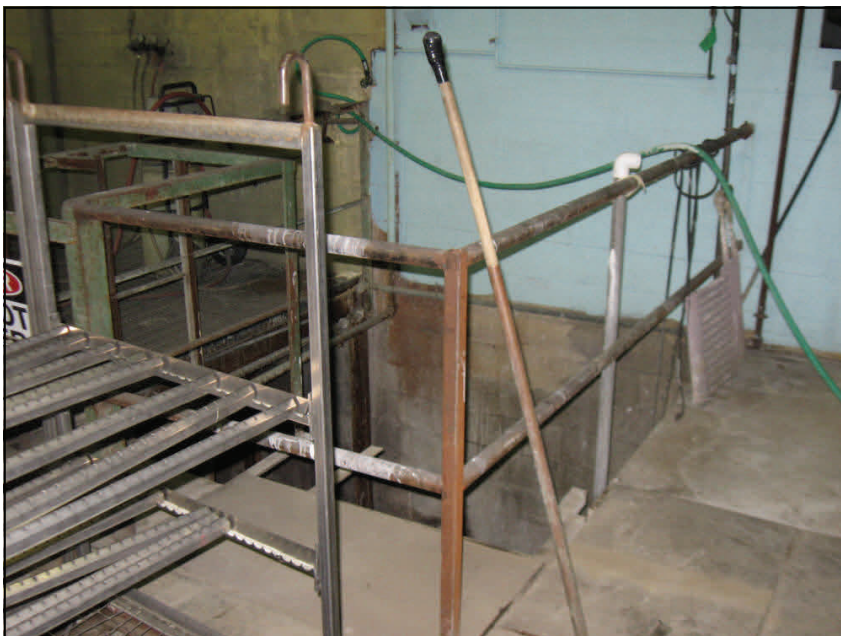
Metal finishing process waste water and pollutants were directly discharged into the sewer system/drains from overflows and direct discharges from the pit area shown above.
