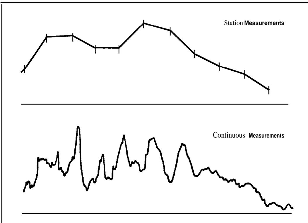
Figure 1-3 Discrete sampling versus continuous geophysical measurements (from Benson et al., 1984a).
