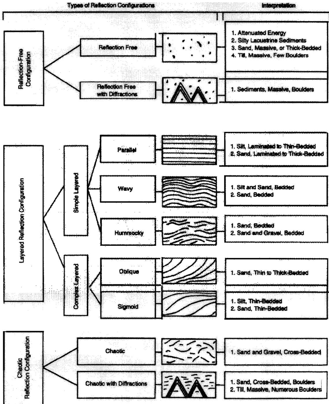
Figure 6-2 Reflection configurations on ground penetrating radar images indicating the lithologic and stratigraphic properties of sediments in the glaciated Northwest (Beres and Haeni, 1991).
