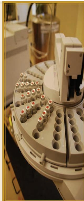
The Region 3 Laboratory conducts testing for a variety of environmental samples, including drinking water, surface water, air, soil, sediment, tissues, and waste drum samples. Specific services and information on submitting samples to the laboratory are available on the [lab services website](#).
