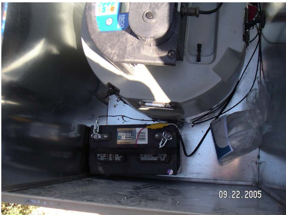
Photo 12. Meadows Detention Basin - marine battery in sampler.
