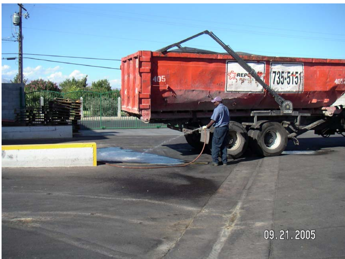
Photo 2. Roll-off container is leaking.
