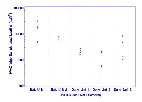
Figure 5-1. Lead Loadings (μg/ft²) Within Wipe Dust Samples Collected from Inside HVAC Ductwork in the R&R Study (Source: USEPA, 1997)
