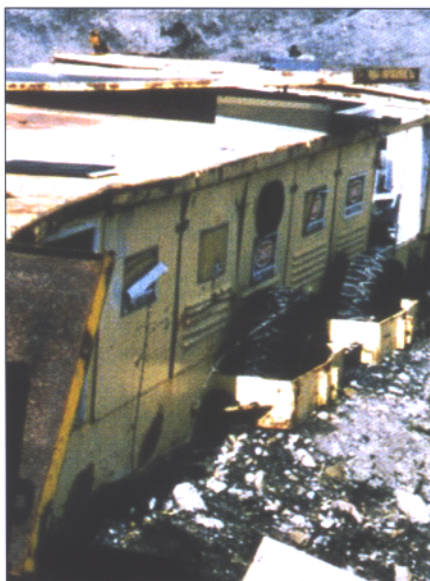
Mine Power Center Commonly Containing Capacitors
