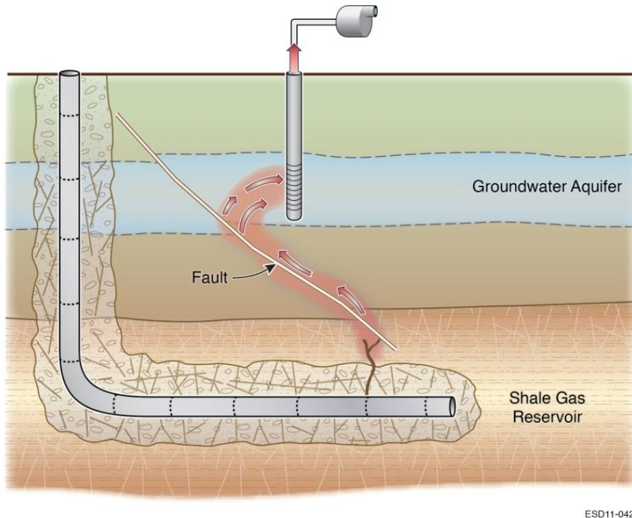
**Figure 5.** HF hypothetical failure scenario E.
