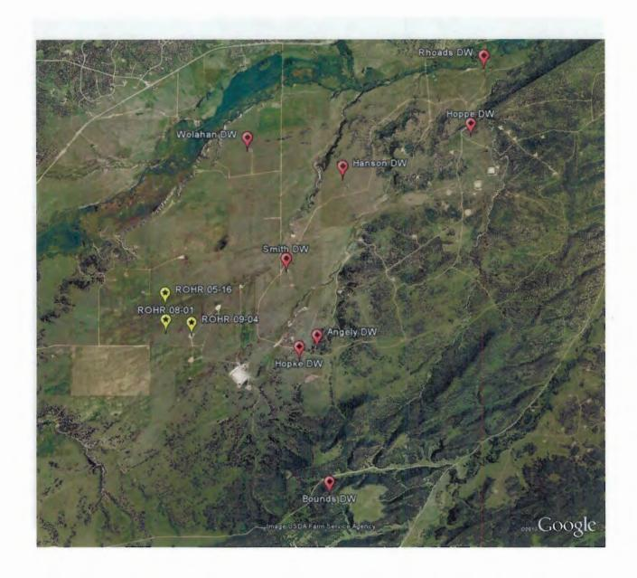
Figure 5. Little Creek Area (Site 2 on Figure 2). Red symbols (diamonds) domestic wells. Yellow symbols show the locations of three stimulated wells (gel fracs).
