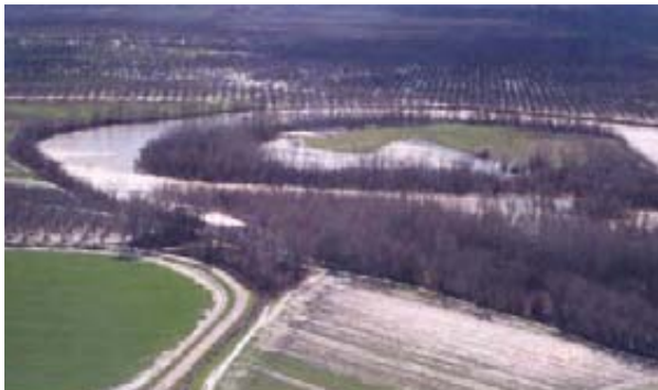
The SPFC relies on the Three B's Natural Overflow Area to protect downstream levees on the Sacramento River
